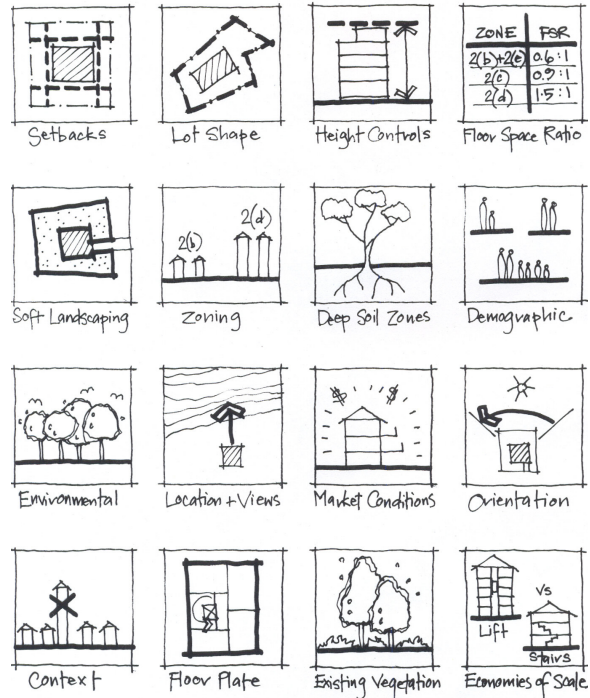
Example of variables which may affect the achievable density for a site.
